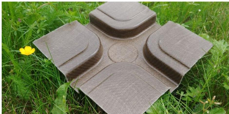
Demonstrator component with polylactic acid matrix and fabric reinforcement based on flax fibres. The component surface features a brownish bio-carbon appearance, which comes from the flax fibres.
