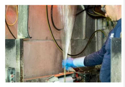
The use of LANXESS Trixene Aqua BI 202 can improve the strength of glass strands and impart composites higher mechanical, flexural properties, as well as improve impact resistance. Photo: LANXESS AG
