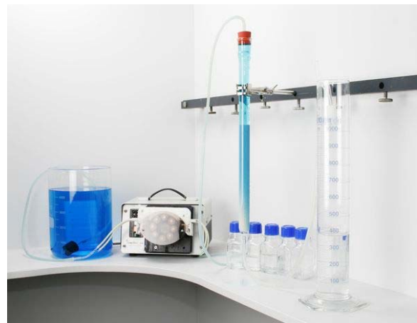
figure 4: It does not take much to test ion exchange resins in laboratory scale. A pump and a glass-column are most important. The rest is standard equipment.
