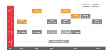
The Pocan XHR product variants achieve Class 4 or even Class 5, the two highest gradings in the USCAR tests. Photo: LANXESS AG
