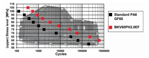
In the HiAnt fatigue screening test, Durethan BKV60PH2.0EF is partly many times more resistant to cyclical mechanical loads than the standard product with the same glass fiber content. Photo: LANXESS AG
