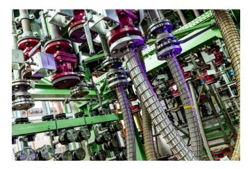
The equipment of the new production line in the ZeTO can be flexibly connected via tube stations. Photo: Saltigo GmbH
