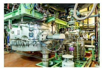
The hydrogenation products are isolated and purified, for example, in the distillation plant connected by a pipe bridge or via crystallization and solids isolation in one of the Saltigo multipurpose plants at the Leverkusen site. The picture shows an eight cubic meter Hastelloy nutsche filter. Photo: Saltigo GmbH
