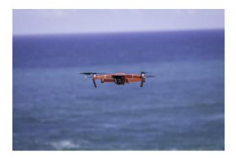
LANXESS's Durethan high-performance plastics are in use for drone propellers but are also suited for drone bodies and landing gear. The materials help to reduce the weight of the aerial vehicle and thus enable longer flight times, as well as reducing vibrations and noise.
