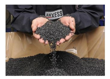
Durethan engineering plastics (PA 6 and PA 6.6 compounds) are used in numerous applications, above all in the automotive industry plus the electrical/electronics sector, but also in the construction industry, in medicine and in sports and leisure products.
