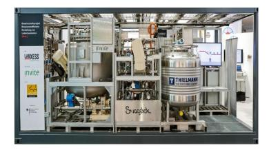
A production plant for resource-efficient production of leather chemicals is debuting this year's Achema. The innovative system for recycling shavings in leather production is designed for use directly on-site at tanneries. Shavings and organic biomass are used to create "X-Biomer" brand retanning agents for manufacturing leather. Photo: LANXESS AG
