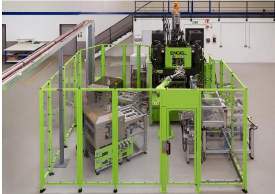
Demonstration cell for processing Tepex continuous-fiber-reinforced thermoplastic composites at Bond-Laminates. Tepex can be shaped in a fully automated process that resembles actual production conditions, and also shaped and oversprayed simultaneously in a hybrid molding process. Photo: LANXESS AG
