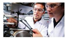
Marked specimens of the new, halogen-free, flame-retardant polyamide Durethan BKV45FN04 are clamped in a tensile testing machine. Photo: LANXESS AG
