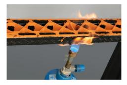
LANXESS' own fire test on a model carrier: The black carrier profile is made of one of the new Tepex grades, the rib structure of an orange, likewise halogen-free flame-retardant polyamide 6 Durethan. The flames do not spread, but extinguish when the burner is removed – regardless of whether the carrier is flamed over the surface or at the edges.
